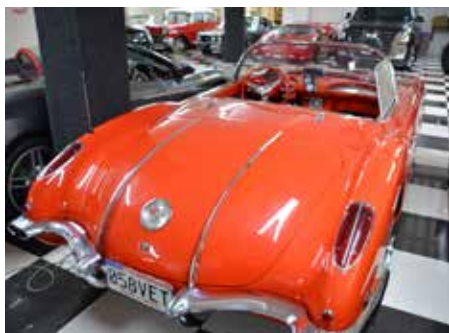
1958 Corvette; note tail pipes in the bumper
