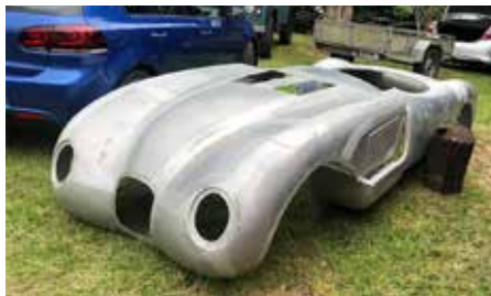
Stunning Jaguar C Type body in bare metal aluminium
