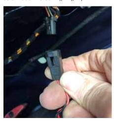
xiv) cable connector releasing intermediate loom
