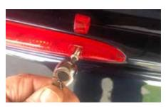
iv) removing LED unit fixing screws with torx ratchet
