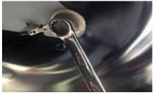
xv) releasing earth cable of intermediate loom
