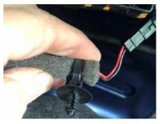
xiii) released mushroom clip and intermediate loom (foam wrapped). Note cable connector clip at top right of frame.
