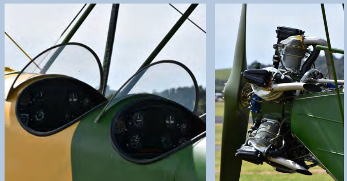
Tiny open cockpit of WW1 fighter. (right) Extraordinarily complex radial air-cooled engine technology of WW1 aircraft
